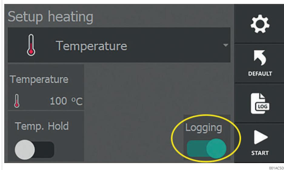
1. Press the [Logging] selector switch to activate the log function.
