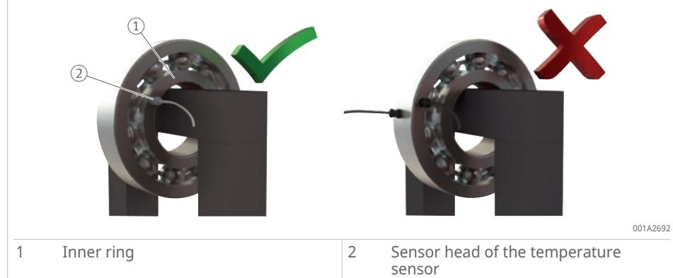
The following should also be observed for heating methods involving a dual temperature measurement or for monitoring by means of the Delta T function:
