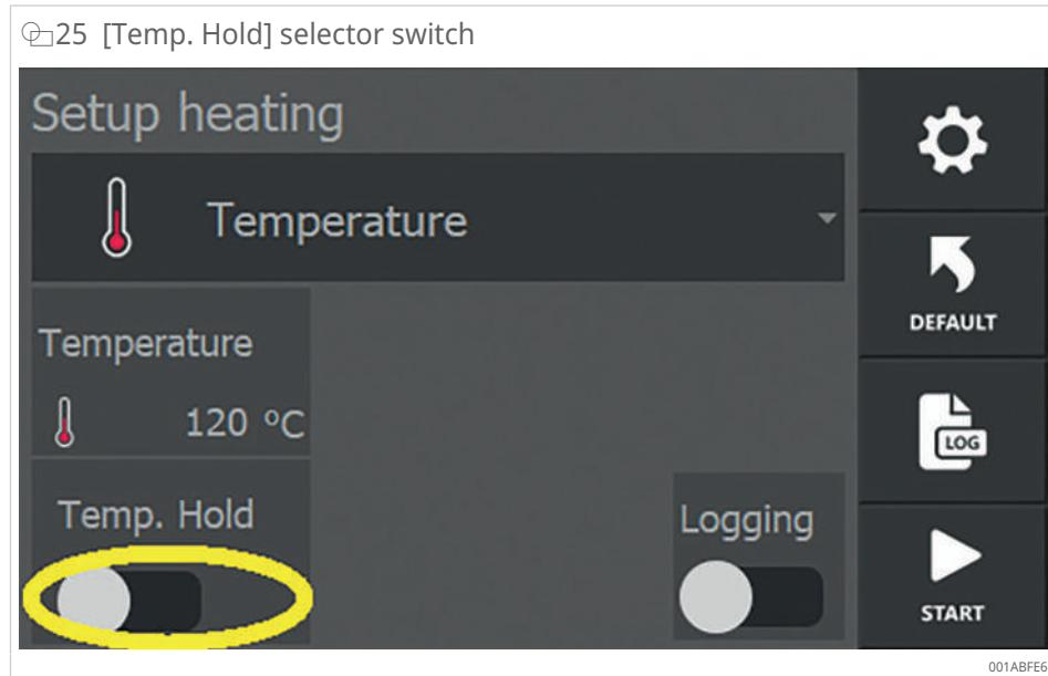
The temperature is held at a specific temperature with a switching hysteresis, which is set in the system settings. The temperature to which a workpiece can fall before the heater is automatically reactivated is set in the system settings.
