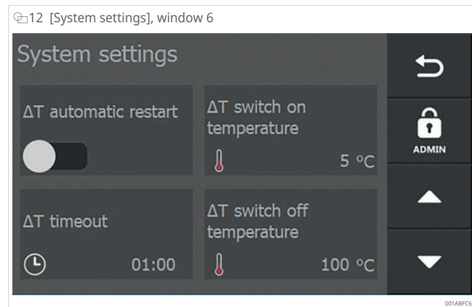
Window 6 is only displayed if the [Enable  $\Delta T$ ] selector switch has been activated in window 5.
