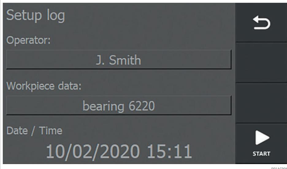
8. Heating can start once all input fields have been completed.
